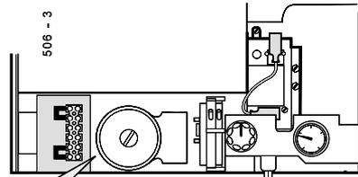
Rotate the restrictor handle anti-clockwise to increase temperature and clockwise to decrease temperature as indicated on the handle.
